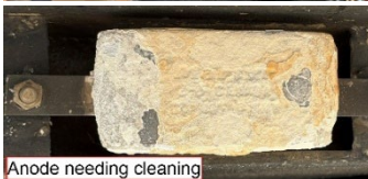
Anode needing cleaning
