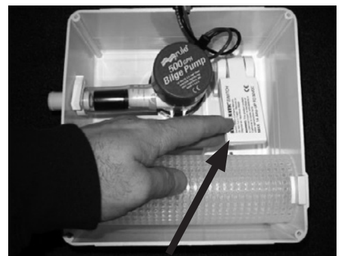
Tripping the float switch
