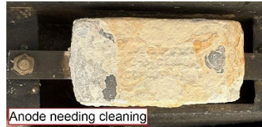
Anode needing cleaning
