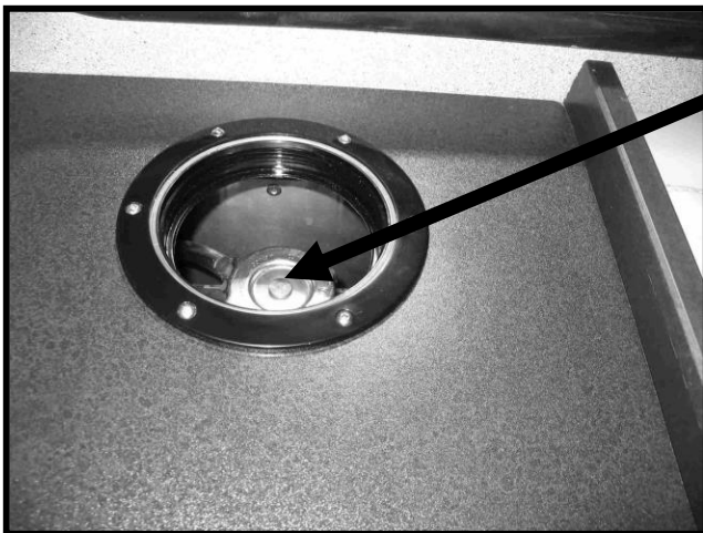
Reservoir Tank Fill Cap
