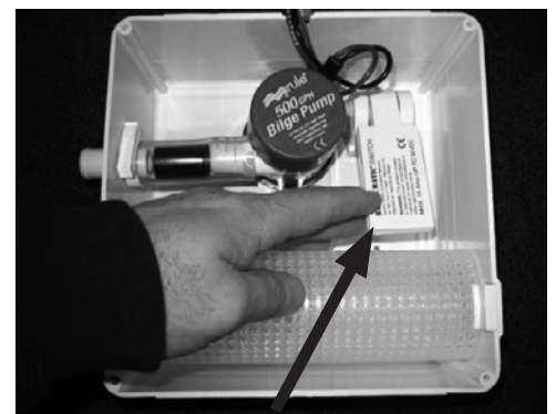
Tripping the float switch
