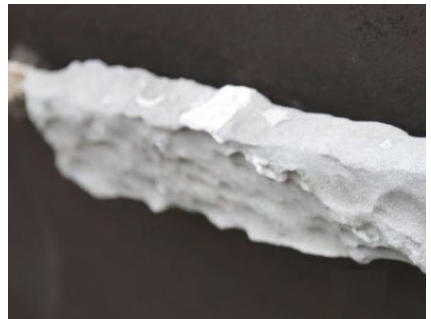
Anode Needing Replacement
